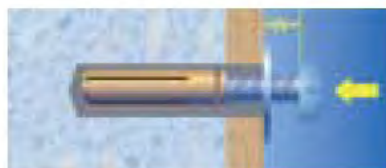
Insert dowel with screwed-in screw into drill hole
