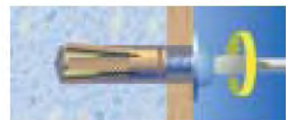
Spreading the anchor by tightening the screw
